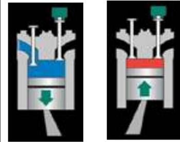
(2) Air is compressed by the engine piston. The energy required to compress this air is produced by the vehicle's driving wheels.
