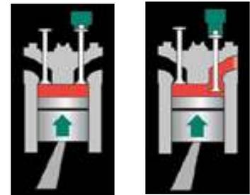
(3A) On the downward stroke, essentially no energy is returned to the piston (and to the driving wheels). There is a loss of energy. This loss is how the retarding work is done.
