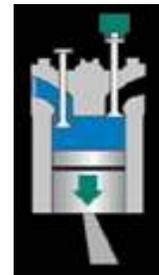
(2A) Air is compressed to approximately 500PSI by the engine piston. The energy required to compress this air is produced by the vehicle's driving wheels. Near top dead center, the Jacobs Engine Brake® opens the exhaust valves, venting the high pressure air and dissipating the stored energy through the exhaust system.
