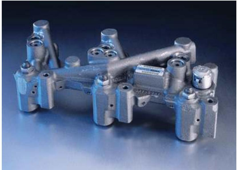
A Jake Brake modifies the timing on the exhaust valves so that, when braking is desired, the exhaust valves open right as the piston reaches the top of the compression stroke. The energy gathered in the compressed air is released, so the compression stroke actually provides braking power.
